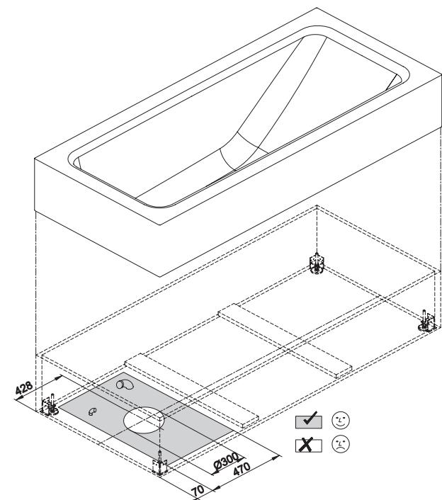
Adequate position to connect the drainage
